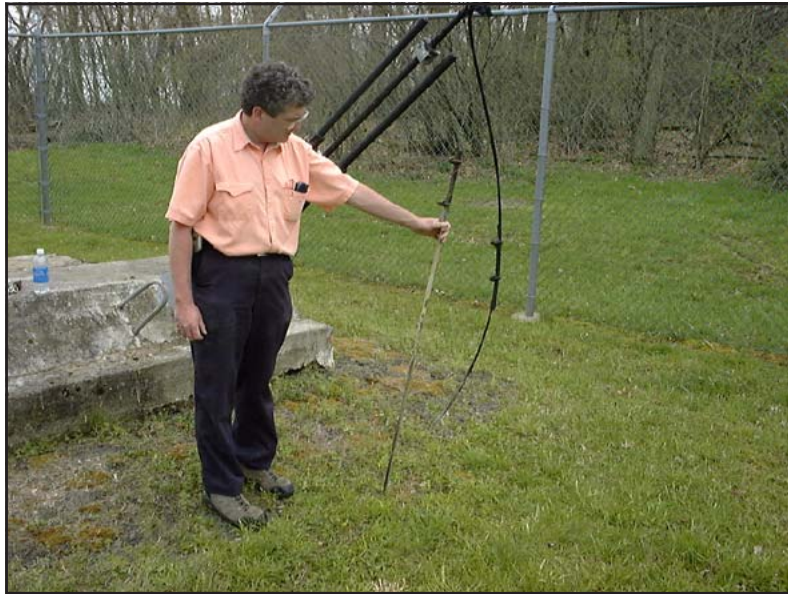
"Joe Wilcher, Maintenance Technician at WTAE TV4, holds one of the 10 pound ground rods that were removed. The ground cable from the guy wires hangs loose near by."
